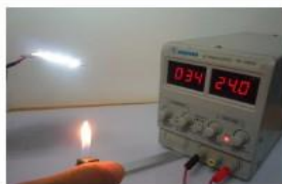
34mA Current when temperature get up
