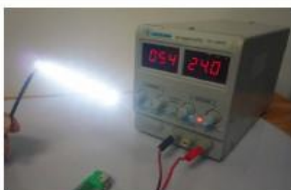
54mA Current before heating
