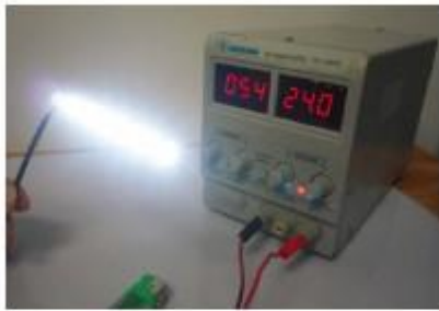
54mA Current before heating
