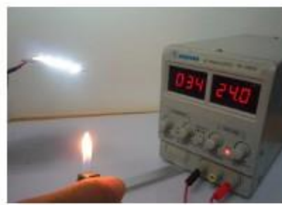
34mA Current when temperature get up
