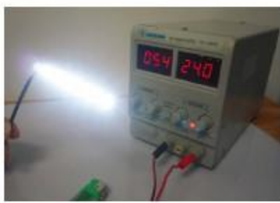
54mA Current before heating
