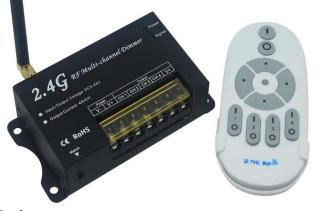
Working temperature: -20-60 °C Supply voltage: 12V~24VDC Output: 4 channels Connecting mode: common anode Output current: 4A Output power: 12V<144W, 24V<288W
