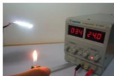
34mA Current when temperature get up
