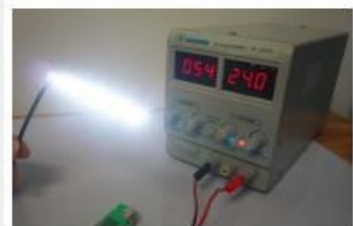
54mA Current when temperature get down back
