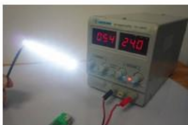
54mA Current before heating
