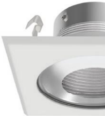
BS4701 4" Square Shower Baffle Trim with Frosted Lens Clear in Centre Lamp: R20/PAR20 LED E26 10W Max. Gasket used to prevent moisture Wet location listed
