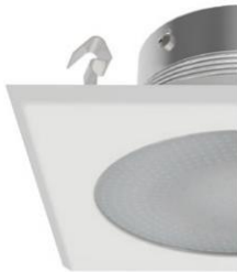
BS4401 4" Square Shower Baffle Trim with Albalite Lens Lamp: R20/PAR20 LED E26 8W Max. Gasket used to prevent moisture Wet location listed
