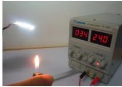
34mA Current when temperature get up
