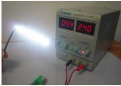
54mA Current before heating
