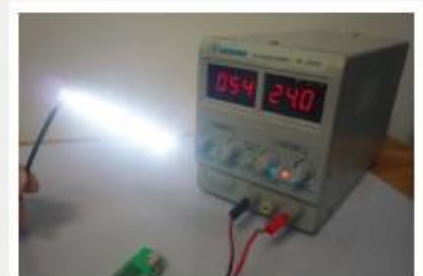
54mA Current when temperature get down back
