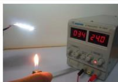
34mA Current when temperature get up
