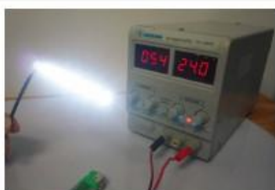
54mA Current before heating
